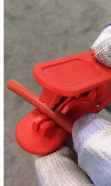
Figure 8-11 Cutting off the end of the fire-trace tube
