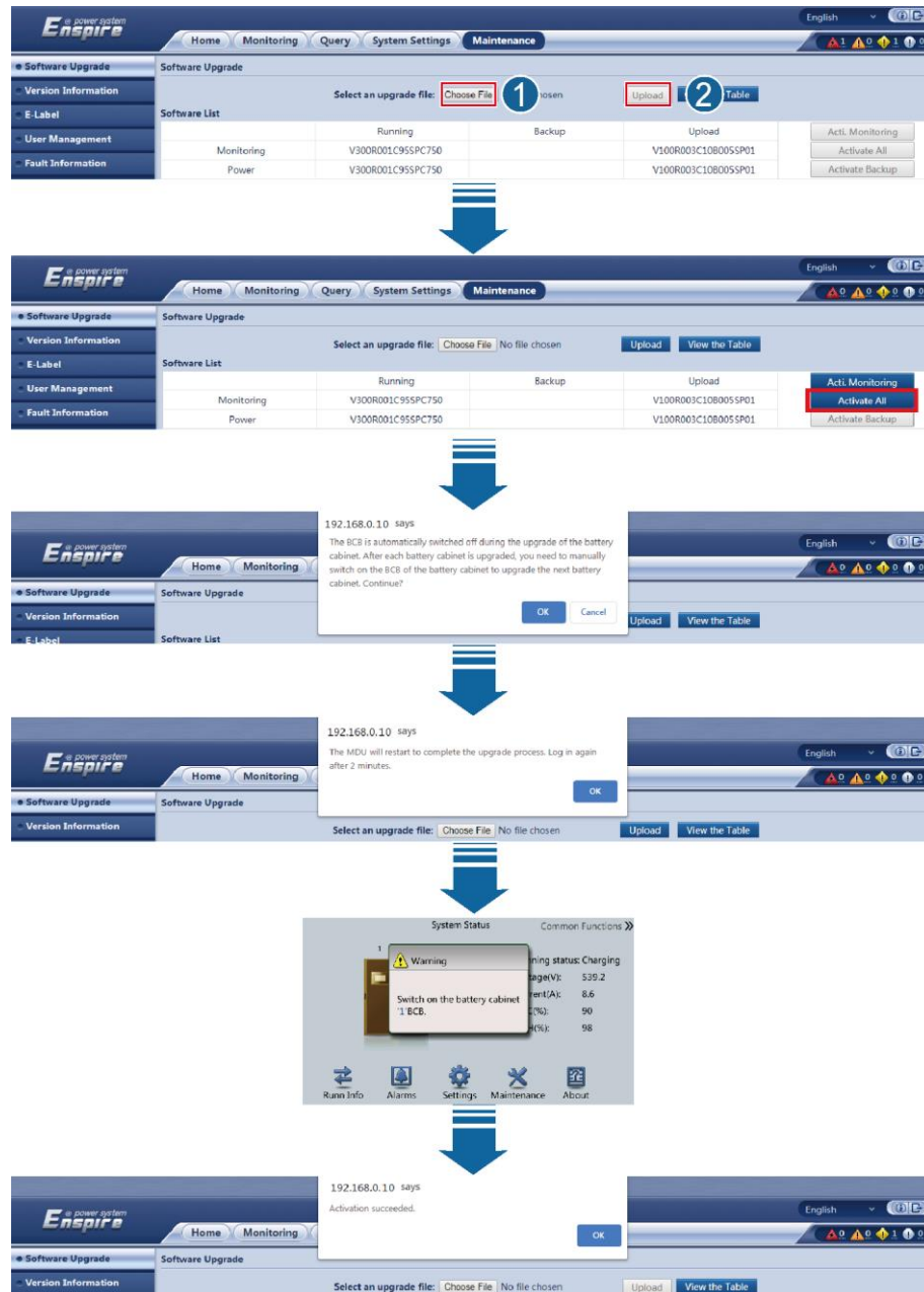
Figure 8-1 Uploading and activating the software (the BCB switches of all battery cabinets are ON)
