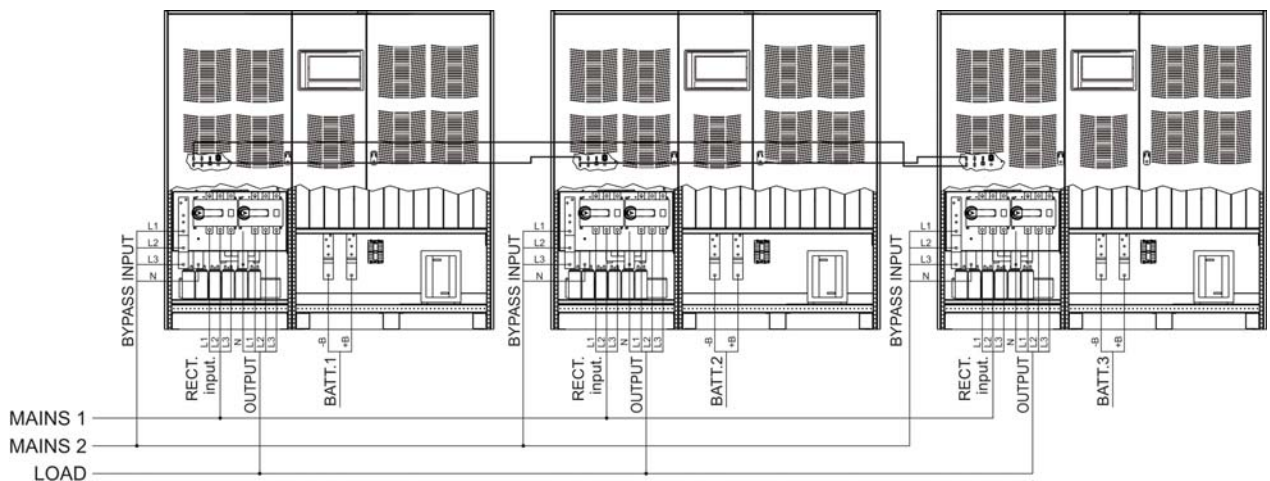
Picture 22 – Connection UPS 3 units 500kVA
