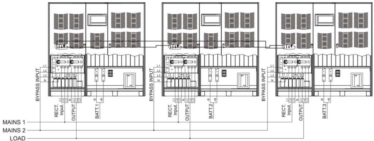
Picture 12 – Connection UPS 3 units 500kVA
