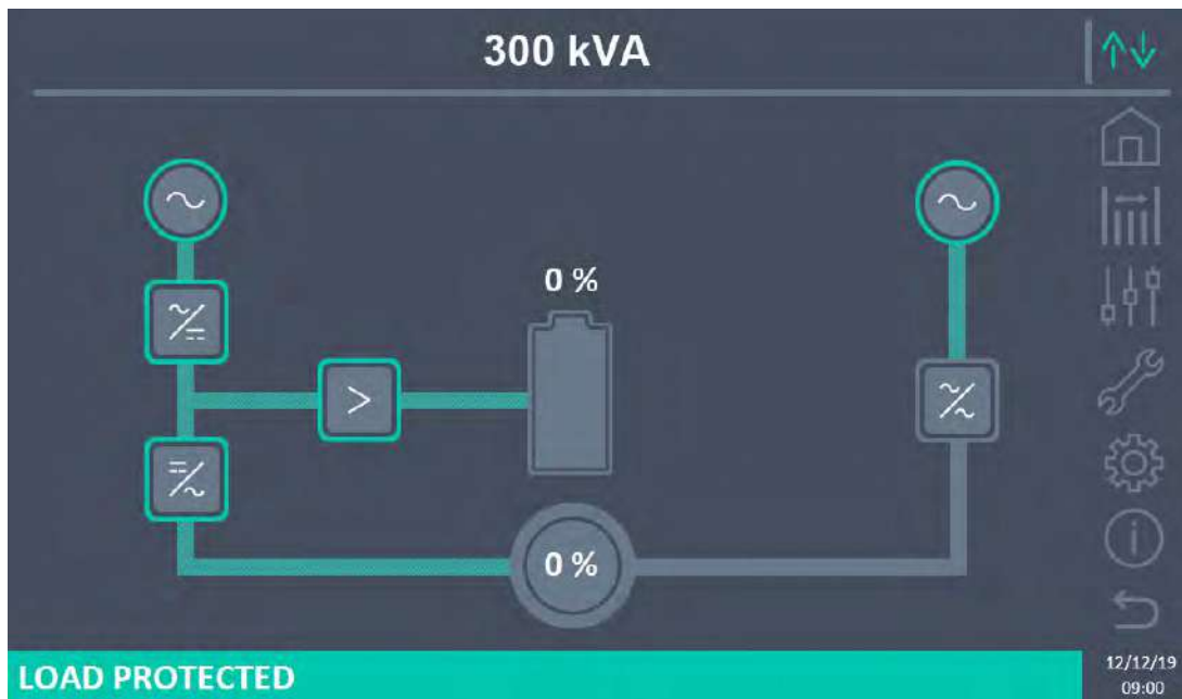
Picture 25 – Re-start from manual bypass completed
